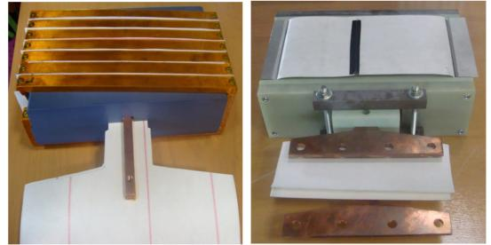
Figure 6: Assembly of the uniform pressure actuator. Left: Coil with core. Right: Complete coil with housing and conductive channel
