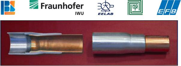
Figure 16: Electromagnetic pulse weld of an aluminium to a copper tube (Source: Pulsar)
