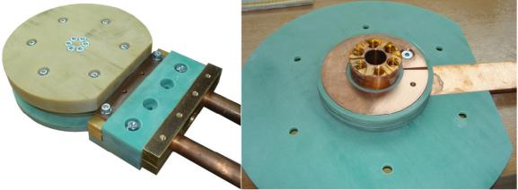
Figure 5: Left: Assembled cutting coil with feedings Right: During assembly
