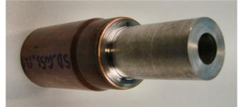
Figure 20: Copper-steel weld (tube diameter: 25 mm, wall thickness: 1,5 mm)
