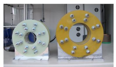
Figure 8: Left: New designed Bitter Coil - Right: Existing BWI Bitter coil
