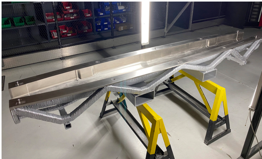
Caption: Lay-up mold for aerospace composite part manufacturing; material: Invar; approximately 200kg and over 3m in length – Courtesy: Lincoln Electric
