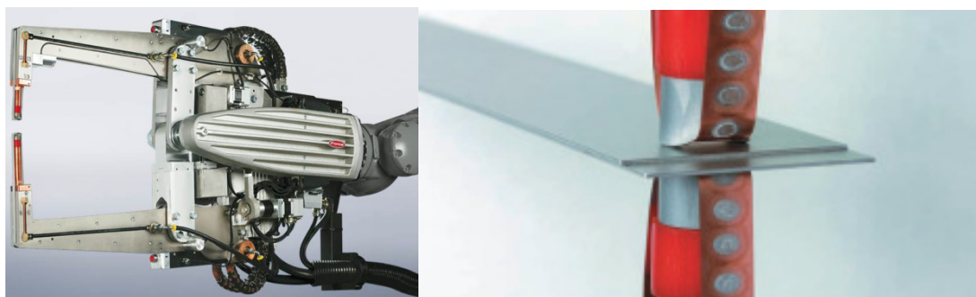
Figure 2: Resistance welding with process tape (Source: KULeuven)
