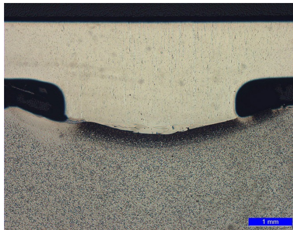
Figure 26: Cross section of the auxiliary joining part (element) welded onto the bottom sheet
