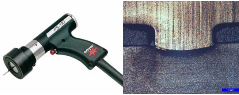
Figure 24: Arc element weld with an auxiliary joining part (Source : Soyer / SLV)
