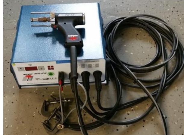
Figure 34: Stud weld device and weld gun at SLV Halle
