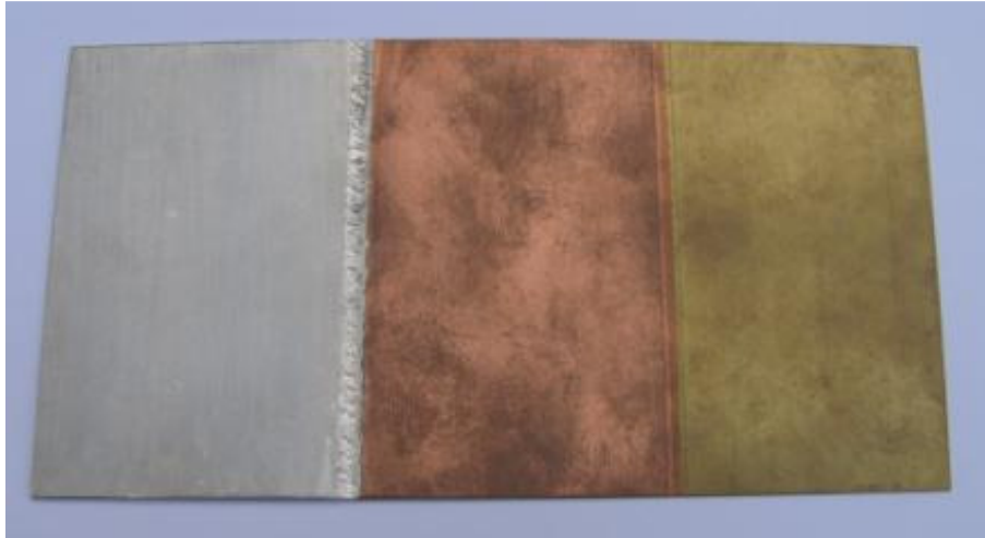
Figure 14: Friction stir welding of copper to brass to aluminium (sheet thickness = 0,5 and 0,8 mm) (source: CEWAC)
