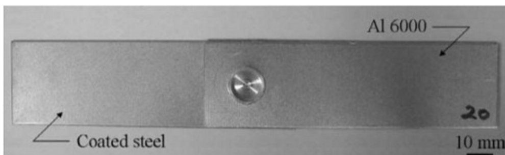
Figure 10: Example of a friction spot weld of aluminium to steel (Source: SLV)
