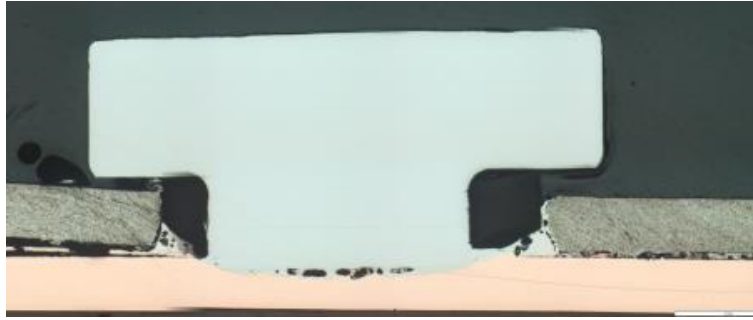
Figure 53: Arc element weld of copper to aluminium (Source: SLV)
