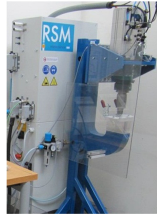
Figure 31: Friction element welding machine at LWF
