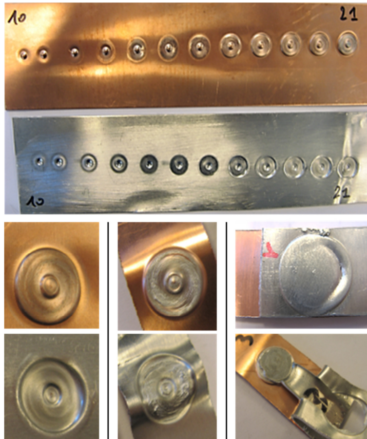
Figure 48: Increasing strength of the Cu-Al FSSW joints, obtained during experiments with copper on top (from left to right), going from Cu & Al deformation without any adhesion up to tearing out of the weld nugget (Source: CEWAC)
