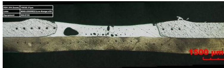
Figure 44: Resistance welding with process tape of copper to aluminium (Source: KULeuven)
