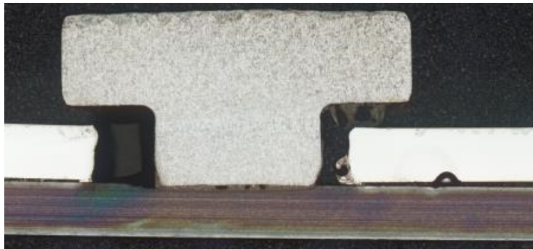
Figure 58: Arc element weld of high strength steel to stainless steel (Source: SLV)
