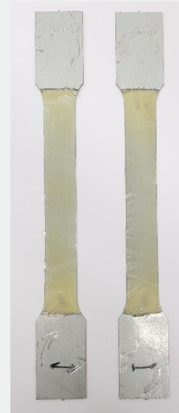
Specimen for tensile test (Litecor 1.3 mm)
