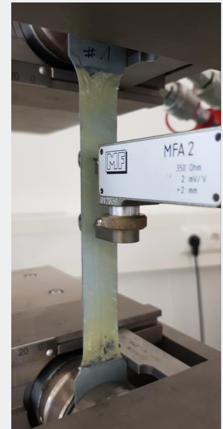
Test setup, strain extensometer
