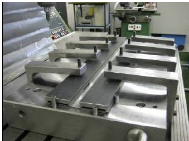
Figure 40: Clamping device for \mu FSW 0,8 mm thick 5754-H111 alloy.
