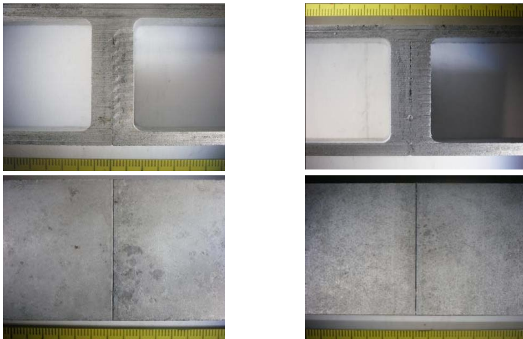
Figure 14: Results of de-icing salt corrosion testing. Left: sample from U3; Right: sample from U4. Top: side view; Bottom: view on the face exposed to the solution.
