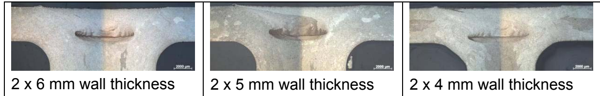
Figure 12: Keller's mod. etched macrographs of friction stir welds realised by CEWAC with C2 welding parameters.
