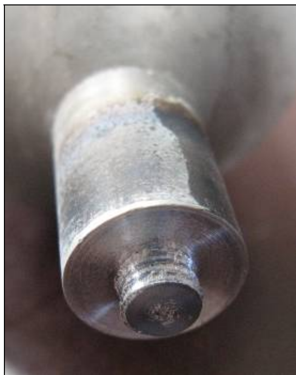
Figure 10: Friction stir welding tool used for application 1.
