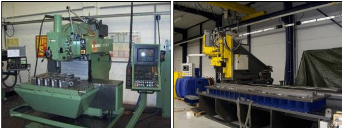
Figure 4: FSW equipment available within CASSTIR. Left: 12 kW HERMLE 3-axis CNC milling machine (UWF 1001 H) at UCL; Right: one of the two ESAB SuperStir™ FSW 53 STL machines at CEWAC.
