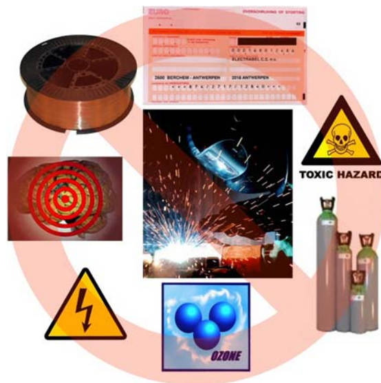
Figure 58: A number of hazards / risks with respect to the environment which are reduced or avoided when applying FSW instead of conventional welding techniques.
