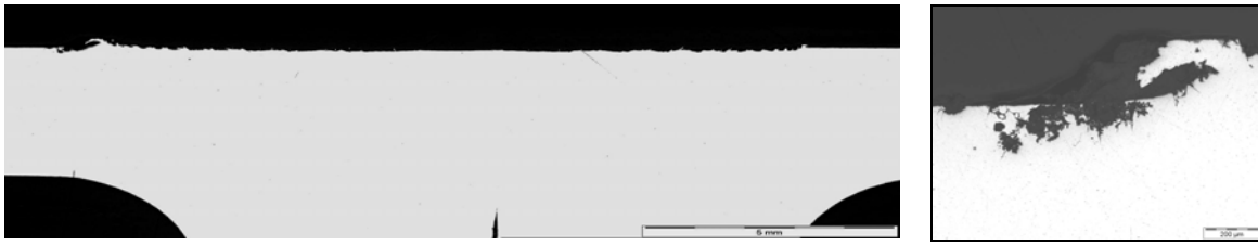
Figure 13: Left: unetched transverse section of a crevice corrosion test sample (weld U4); Right: detail of the HAZ on the advancing side.
