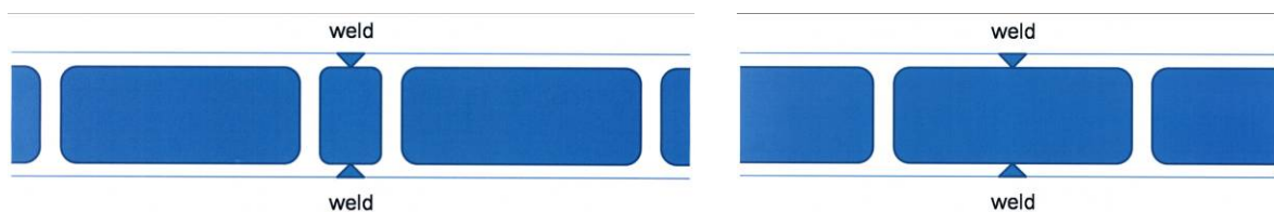
Figure 23: Sketches of alternative extrusion profile geometries considered more suitable for beam welding processes.
