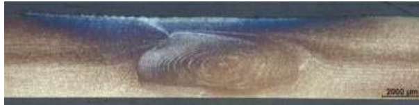
Figure 48: Macrograph of the friction stir weld in 5754-O (4 mm).
