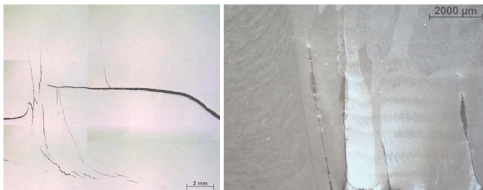
Figure 36: Cracking found in the SHT+AA sample extracted near the end of the weld.
