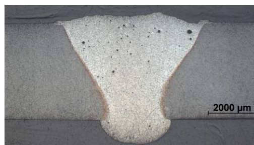
Figure 22: Macrograph of a hybrid laser weld in 6082-T6 flat extrusion profile.
